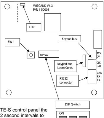
When the RS232 board is connected to an ELITE-S control panel the LED on the board will flash at approximately 1/2 second intervals to show it is working.
